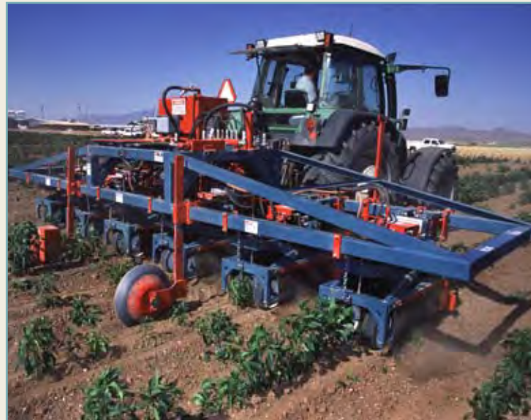
CEMCO designed, and is manufacturing, a totally new machine designed specifically for chile thinning.
